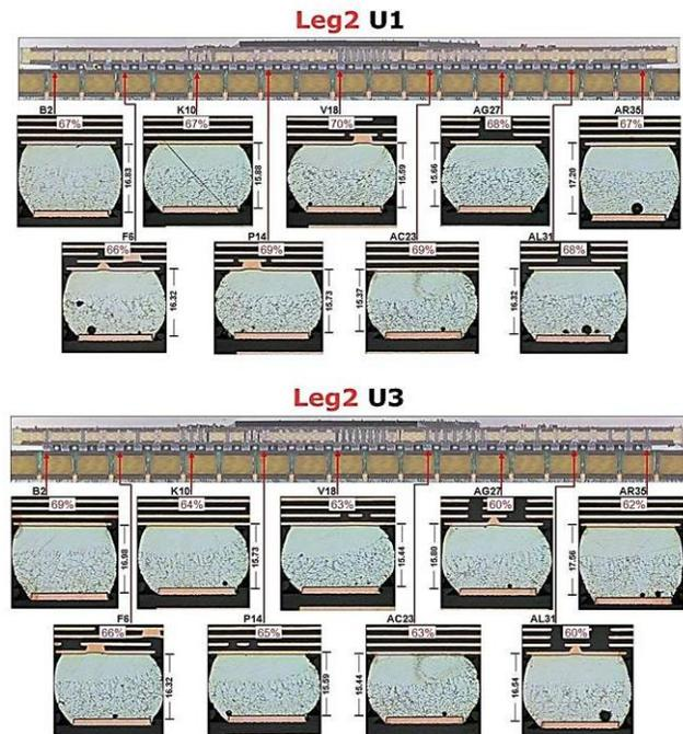
**Figure 4:** Multiple photomicrographs along the diagonals of two Medium Pb mixed, Leg 2 samples. The Pb mixing ranges from 60 to 70% across the diagonal and the Pb mixing is more uniform in the individual balls compared to Leg 1 shown in Figure 3).
