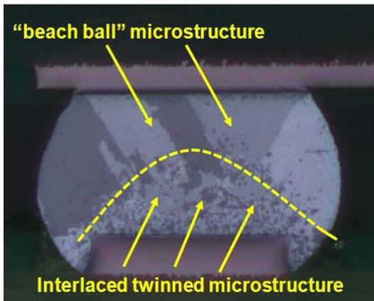
**Figure 15:** A polarized light micrograph illustrating regions that contain beach ball and interlaced twinned microstructures. This image was obtained from a SAC405 sample used in the iNEMI alternative Alloys project [60].
