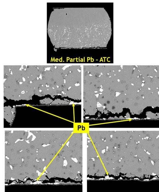
**Figure 11:** Backscattered electron images of thermal fatigue failures at the PCB side of the solder joint in the Medium Pb mixed leg. Note the Pb (bright white phase) accumulated at the soldered interface and along the crack path.
