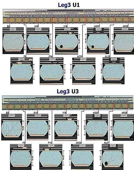
**Figure 5:** Multiple photomicrographs along the diagonals of two Full Pb mixed, Leg 3 samples. Compared to the partially mixed Legs 1 and 2, the standoff height is slightly lower for the fully mixed Leg 3 due to the complete melting and collapse of the solder balls.
