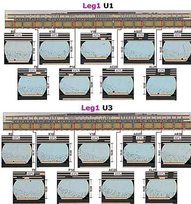
**Figure 3:** Multiple photomicrographs along the diagonals of two Low Pb mixed, Leg 1 samples. The Pb mixing ranges from 40 to 50% across the diagonal and often is not uniform across the solder ball.
