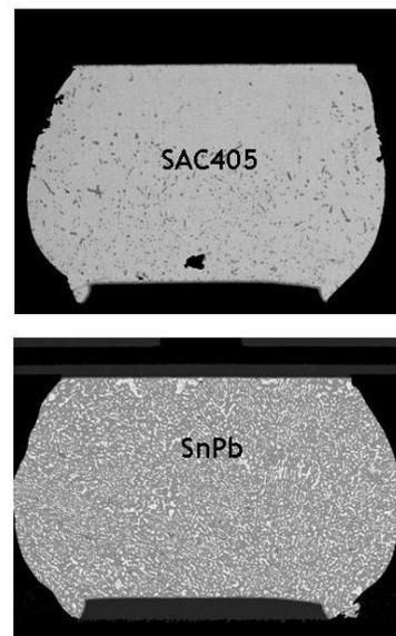
**Figure 7:** Backscattered SEM images for the SAC405 Pb-free and SnPb eutectic control legs. The dark phase in the SAC405 is the  $\text{Cu}_6\text{Sn}_5$  intermetallic; the  $\text{Ag}_3\text{Sn}$  intermetallic particles cannot be resolved at this magnification.
