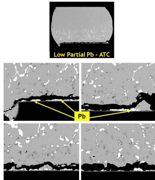
**Figure 10:** Backscattered electron images of thermal fatigue failures at the PCB side of the solder joint in the Low Pb mixed leg. Note the Pb (bright white phase) accumulated at the soldered interface and along the crack path.
