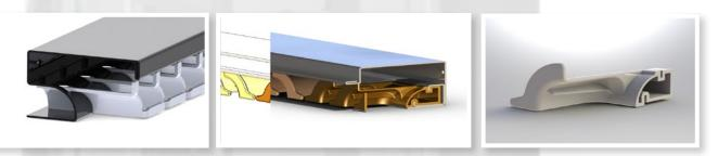
Example 1. Redesign from a welded sheet metal part to a UL-94VO plastic resin molded part, justified thru BDI-DFMA<sup>®</sup> analysis which showed cost savings of 42% per piece.
