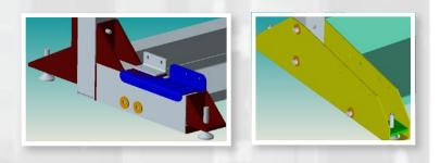
Example 3. Redesign of a frame pedestal foot combining front and back features, which reduced parts from 11 to 5 parts, eliminated other brackets. The hardware reduction went from 5 bolts to 3 bolts. The changes were supported thru BDI-DFMA® analysis which showed projected cost savings of 37%
