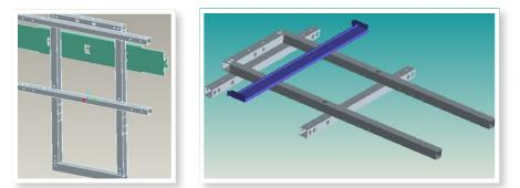
Example 2. Redesigned frame structure from a welded tubing structure to a riveted sheet metal design. BDI DFMA<sup>®</sup> analysis shows cost savings of 58%, significant enough to justify the change.
