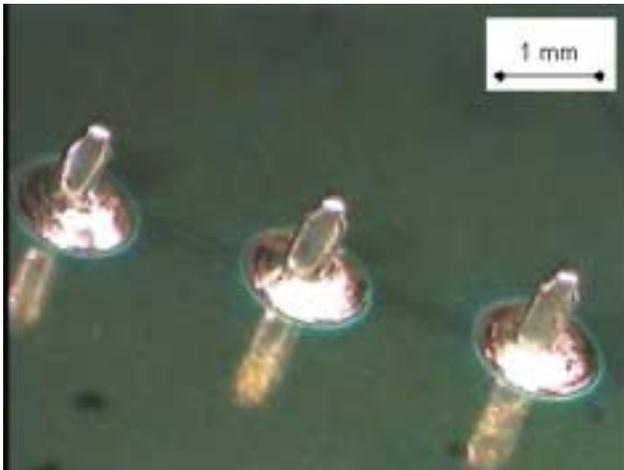
**Figure 16.** Wetting of the solder to the pins on the bottom side of a Sn-Cu/Sn-Bi PDIP assembly.
